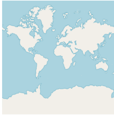
Figure 2. Zoom level 0: The whole earth on a single tile
